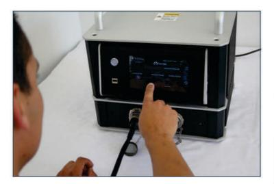
For cables with intermittent performance problems, a real time test mode is offered. This allows the user to monitor either continuity, resistance or insulation integrity while subjecting the cable to mechanical tests.
